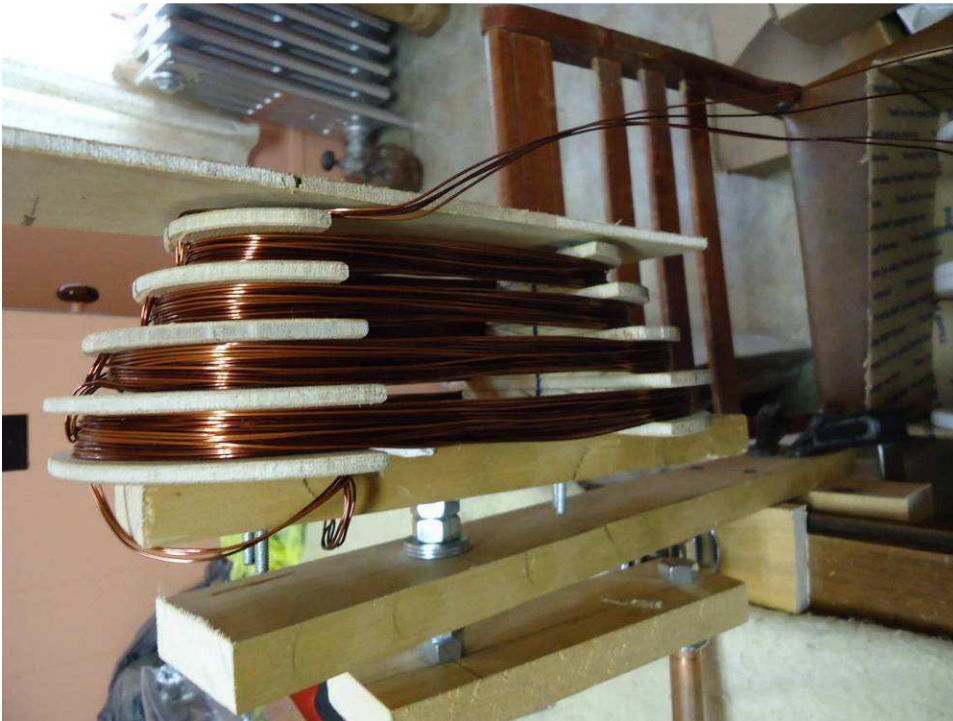
Four of the main winding coils wound. After labeling and removing these completed coils I taped them fast to the board at the front of the winder.
