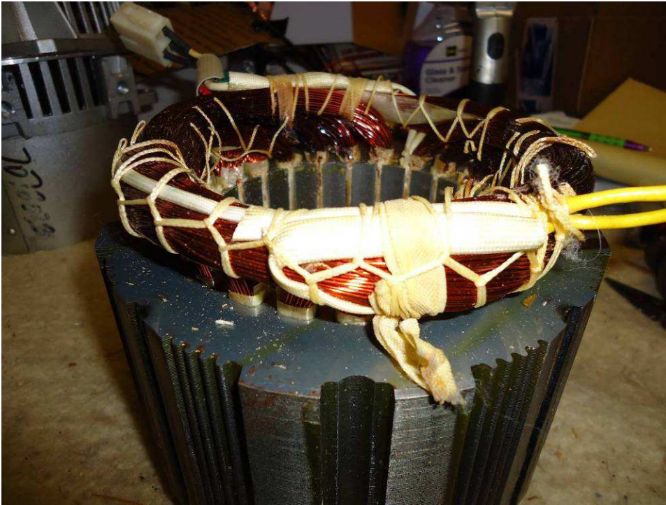
Burnt up 3.5kW generator stator. Notice blackened windings in the back.
