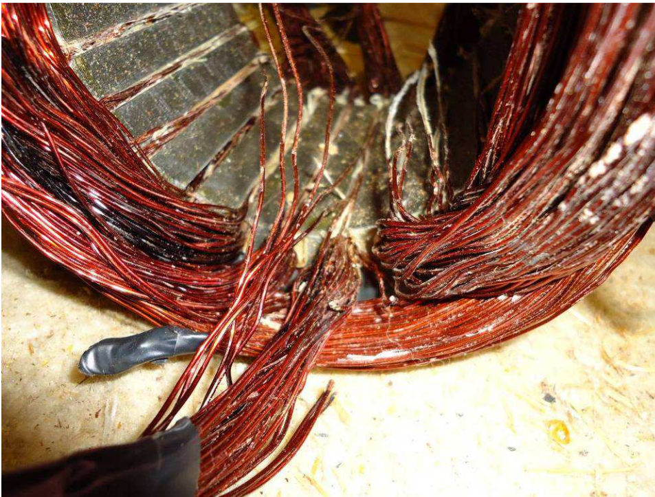
Remove each winding a few wires at a time to fit through the slot openings.
