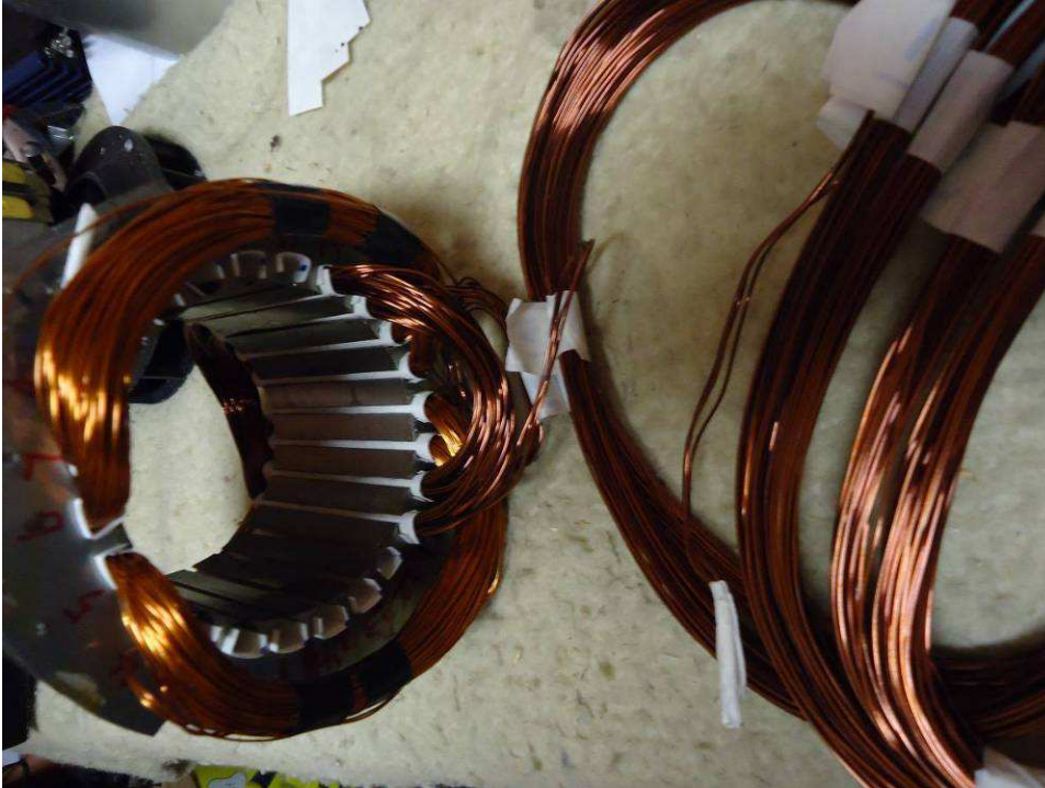
All the Aux. coils installed and the first two coils of the main winding. Note to start with the smaller coil and work to the larger coils.
