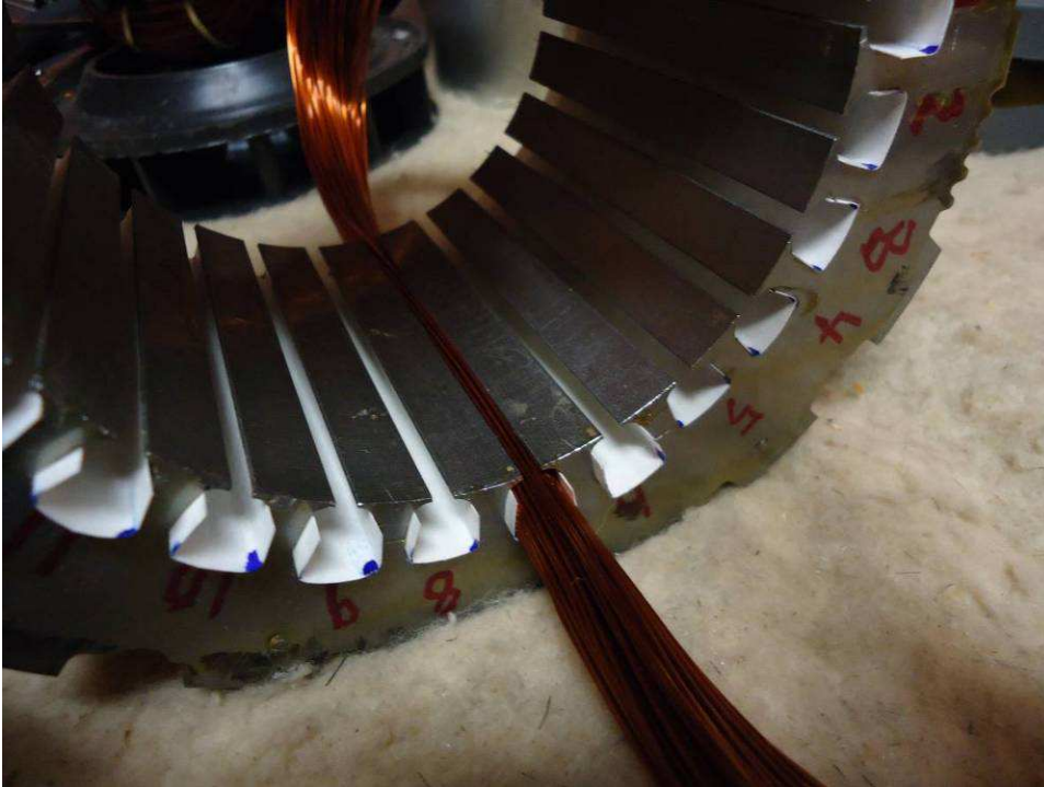
The first coil of the Aux. winding placed into its stator slot.
