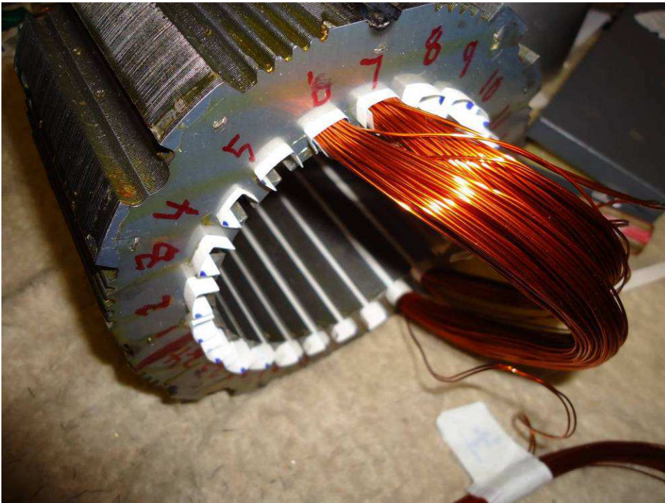
Another photo of the first two Aux. winding coils.
