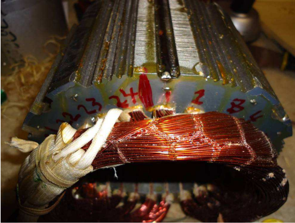
Number the slots so you can document it and put it back together.
